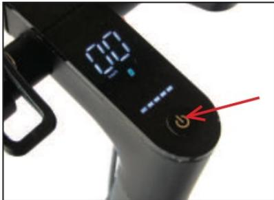
Press and hold the button to turn on the power. The headlights, taillights, and maximum speed indicator light flash.
