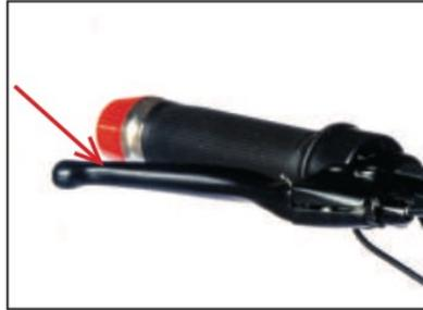
The right handle is the front brake, and the left handle is the rear brake.
