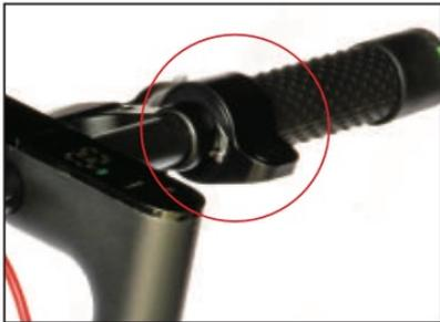
Just like riding a kickboard, kick it out a little and then press the accelerator lever to start driving.
