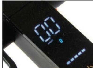
After turning on the power, press the button twice to switch the driving mode.
