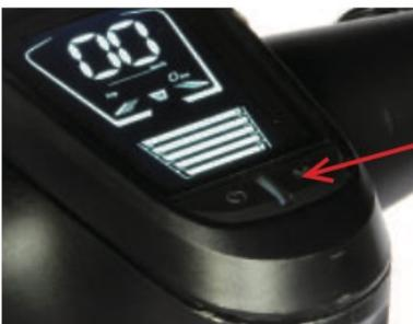
After turning on the power, you can switch the driving mode using the button on the right.
