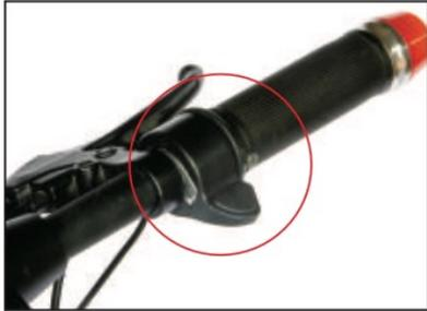
Press the accelerator lever to drive.
